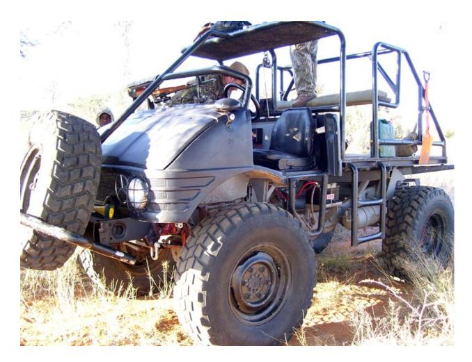
The Unimog is a German product, a sort of general-purpose vehicle with high ground clearance and four-wheel drive, made by Mercedes-Benz. Cornie's was built in 1964 and he took a welding torch to it, cutting off the cab; that was replaced with a roll cage of his own design and construction, and a bench seat in the rear for riders. The original truck bed has been replaced with one of Cornie's design, too.
